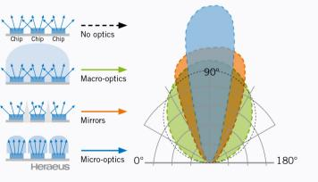
Heraeus unique micro-optics reduce stray light to a minimum with an exit angle of 60 instead of 120 degrees – for all available wavelenghts.
